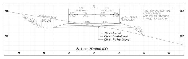
Figure 3.1: Typical Highway Cross Section
